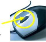
Use of the centre scroll tool on the mouse is also a very convenient method of scrolling in and out.
